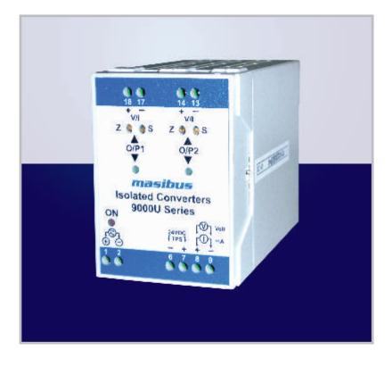
Masibus Signal Isolator Model 9000U is a rugged 4 wire isolator designed to accept custom-built and wide range of voltage and current input signals. Signal is then isolated and converted to standard instrumentation signals, acceptable to commercially off the shelf (COTS) automation products.
