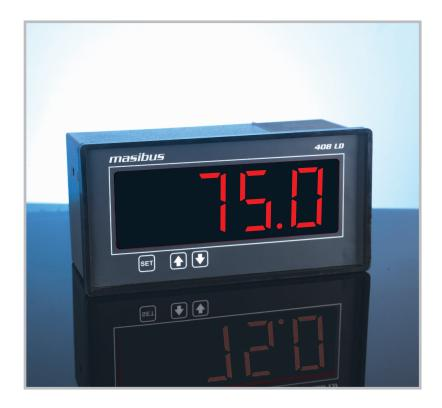
Masibus' large digit display Model 408-2IN accepts universal process inputs. From these inputs the display can be scaled to remotely read in engineering units. Unregulated transmitter power supply is provided as standard on AC supply models.
